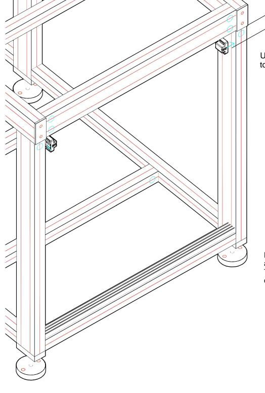
Using drop in t-nuts, install magnet catches on to closest inside slot of leg
