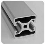
The 1.5" x 1.5"BOS shape was designed for lighter weight and strength requirements where additional cleanliness and aesthetics is needed. Applications include machine enclosures, guarding and light weight frames.
