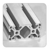
The 1.5" x 3.0"L shape is designed for larger structures where strength is not critical. Applications for 1.5" x 3.0"L include framing and door tracks. This shape can be used to run air lines or as a pressure or vacuum manifold up to  $150 \, \mathrm{p.s.i.}$
