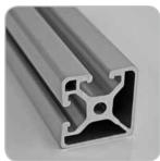
The 1.5" x 1.5"BAS shape was designed for lighter weight and strength requirements where additional cleanliness and aesthetics is needed. Applications include machine enclosures, guarding and light weight frames.
