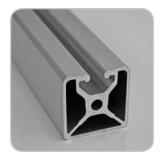
The 1.5" x 1.5"MOS shape was designed for lighter weight and strength requirements where additional cleanliness and aesthetics is needed. Applications include machine enclosures, guarding and light weight frames.
